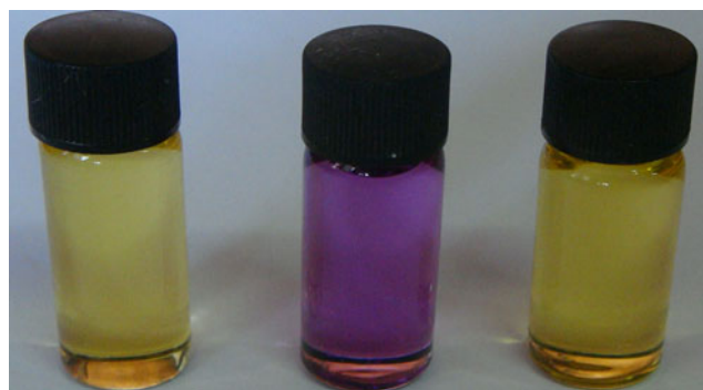
Fig. 2 Color changes of the receptor 1 in DMSO ( 5.0 \times 10^{-4} M) in absence and presence of 10 equiv of anions (from the left to the right: 1 only, 1 + \text{F}^- (the color changes of the \text{AcO}^- and \text{H}_2\text{PO}_4^- is similar with \text{F}^- ), 1 + \text{Cl}^- (the color changes of the \Gamma^- and \text{Br}^- is similar with \text{Cl}^- ))
